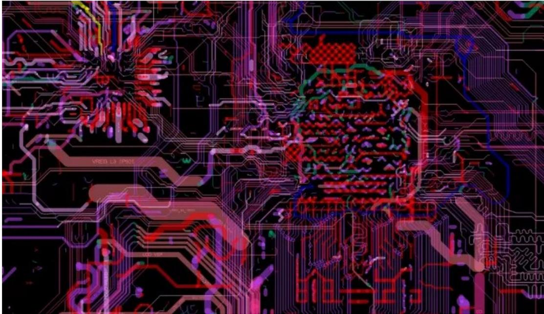
*8-layer 2-step stacked hole, Qualcomm Snapdragon 624 processor PCB*
