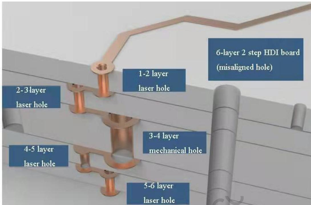
This picture is a six-layer, 2 step HDI board with misaligned laser holes. Usually, people seldom use six-layer 2 step HDI PCB, and most of them start with eight-layer 2 step HDI PCB.
