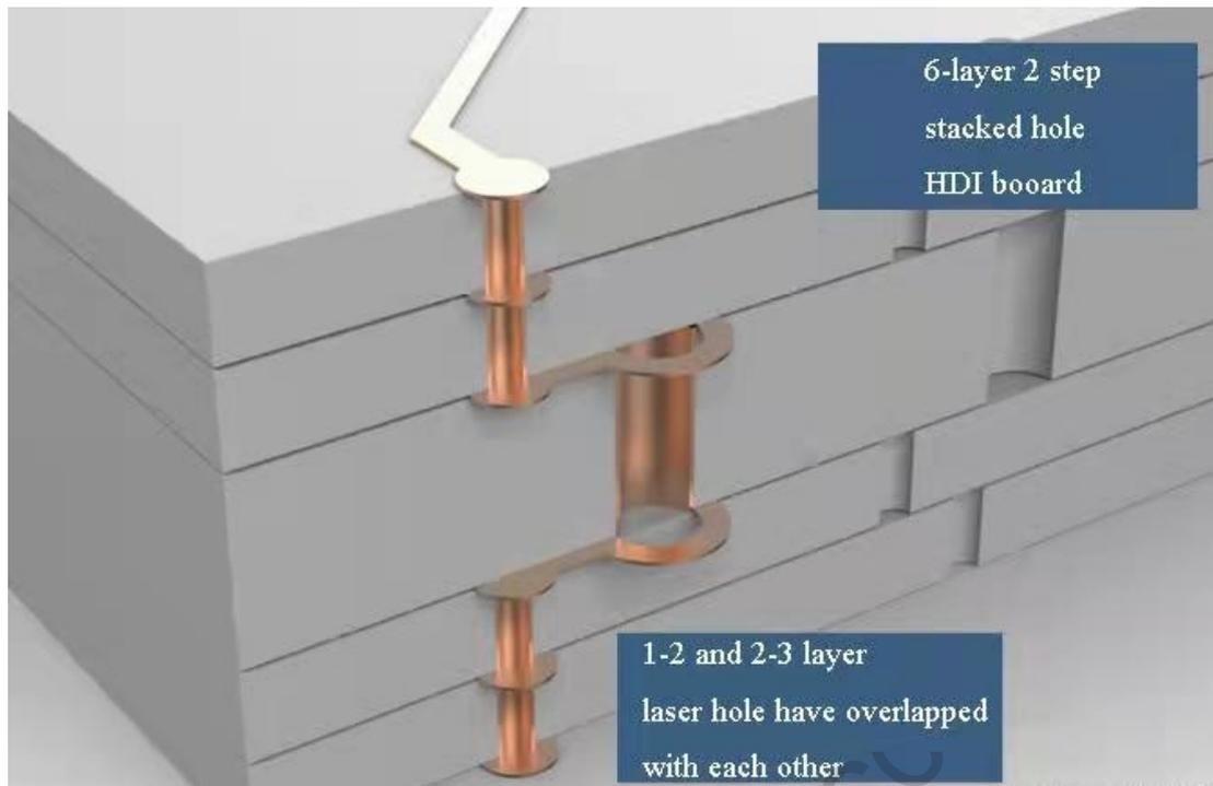
The two layers of laser holes of the stack up hole board overlap each other. The conduct line and components will be more compact.
